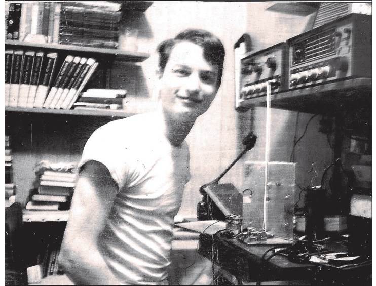
Lenny WB2HKV. The back of the original photo says "April or May '64" which makes the op 15 or 16 years old. Running a rockbound DX60 & matching HR10 with tube based homebrew T-R switch and a homebrew Select-O-Ject active audio filter. A 66 foot dipole standing about 18 inches off the side of the (brick) house struggled to radiate (tho I do have some EU QSL cards from that era). Had lots of fun! At Thomas Jefferson HS (Brooklyn) I operated the club station W2BVH. The Heathkits are still here, down the basement. I'm a real packrat.
